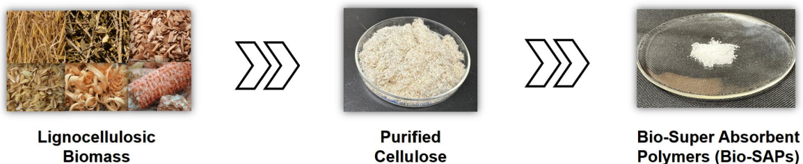
Fig. 1 Production Process of Bio-Super Absorbent Polymers (Bio-SAPs)
